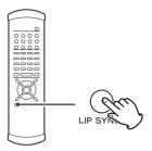
This function allows you to adjust the synchronization of the video and audio portions of a DVD.
